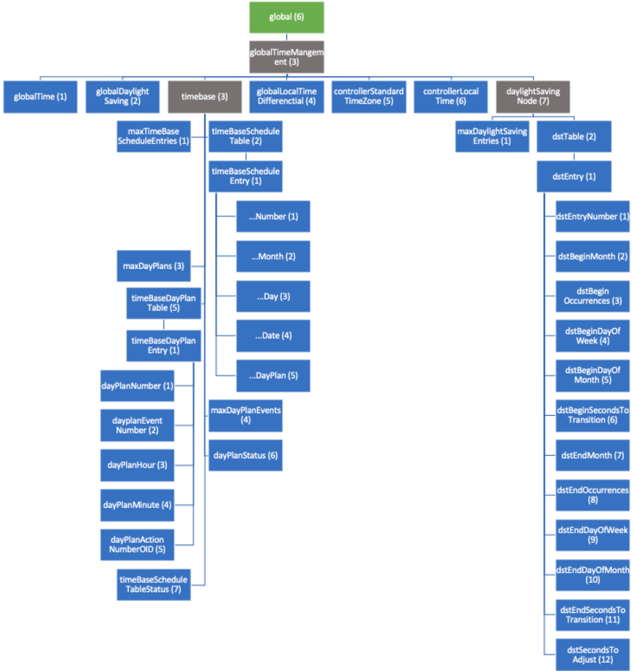
Figure 4: Nodes Defined in NTCIP 1201-Global MIB (Part 2 of 3: Time Management)
