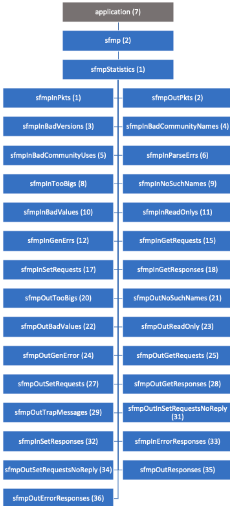
Figure 9: Nodes Defined in NTCIP1201-SFMP MIB
