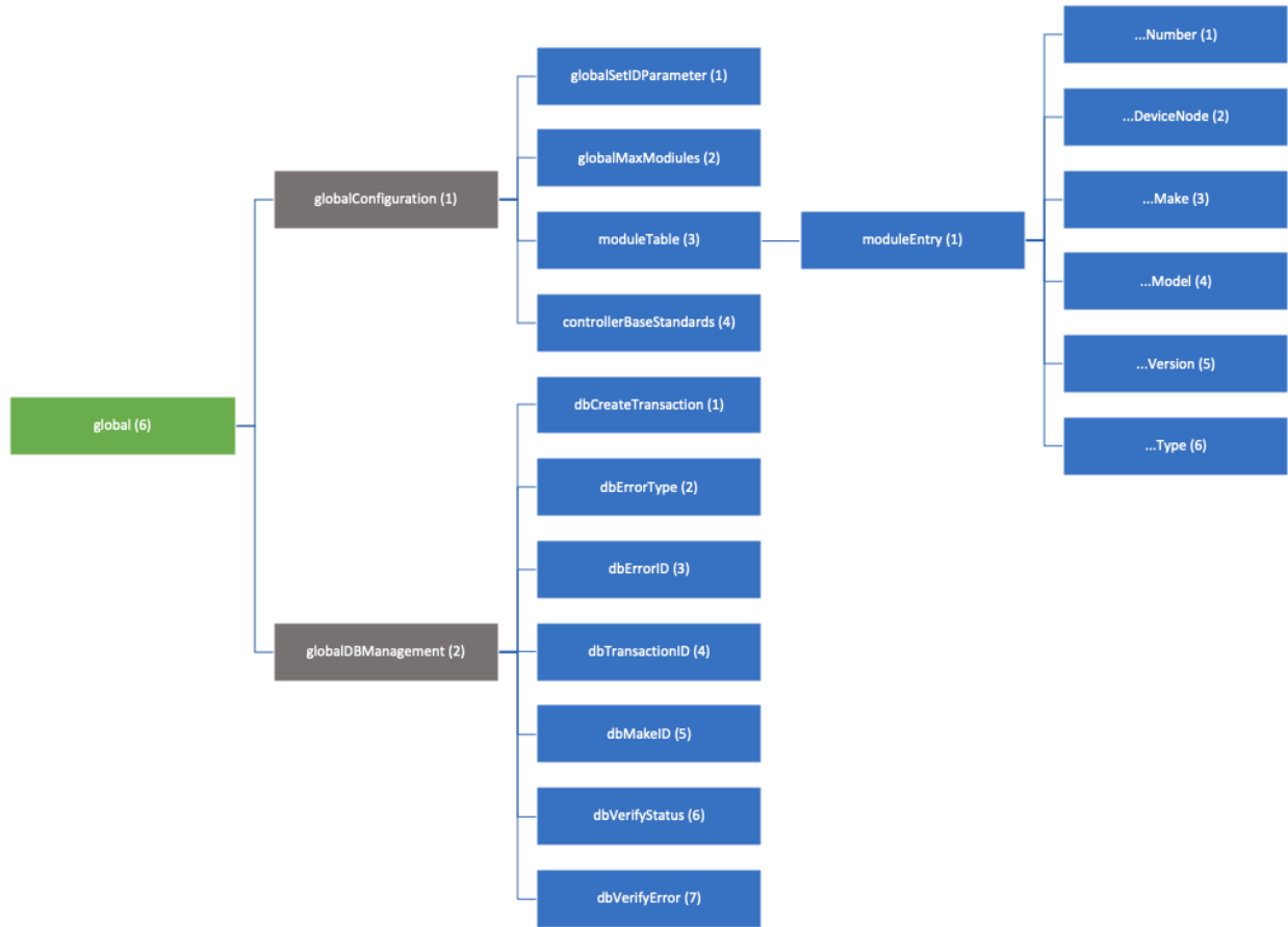
Figure 3: Nodes Defined in NTCIP 1201-Global MIB (Part 1 of 3: Base Objects)
