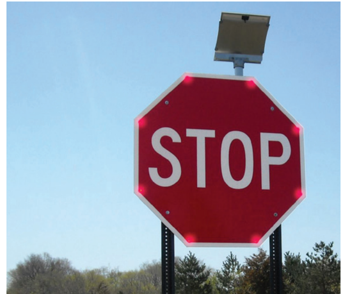
Figure 11. Stop sign with LED enhancement.
