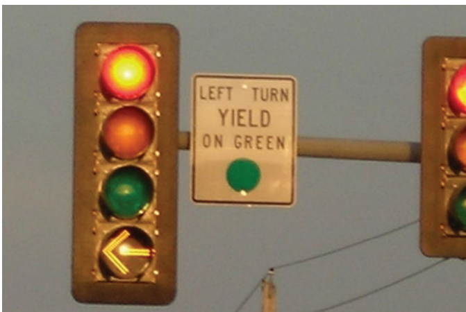
Figure 7. Four-section signal head with yellow indication.
