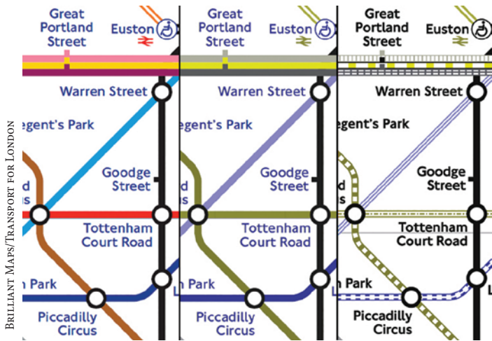
Figure 9. Left: Normal-vision map. Center: Simulated colorblind-vision map. Right: Double-coded map to aid colorblind users.
